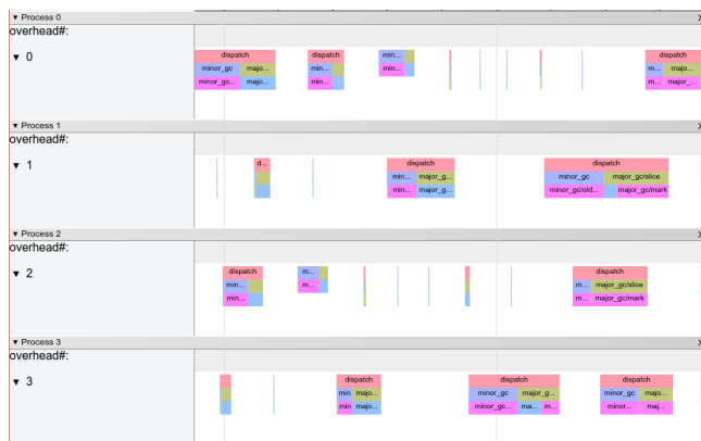
Figure 1. Example eventlog trace from a Multicore OCaml program
